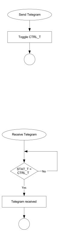
The continuous exchange of telegrams is established. The host application waits for a signal to send a message to the module.
