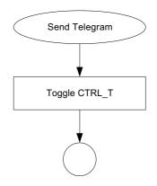
The Anybus CompactCom module checks its status, and when it is satisfied that it has performed all actions possible at the time being, it toggles the STAT\_T bit in Status register to equal CTRL\_T. A valid response telegram is available for the host application.
