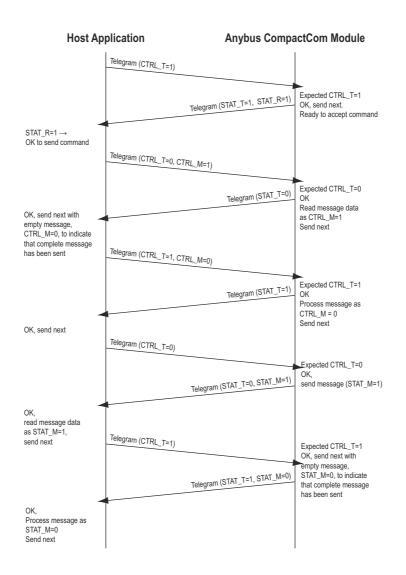
Each arrow in this example of ping-pong communication, indicates a telegram sent either from the application to the Anybus CompactCom module, or the other way around.
