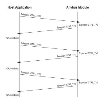
All telegrams, whether in parallel or serial mode, have dedicated sections for control/status information and message data. Once the module is up and running, there is also a section for process data. Telegrams, registers and messages will be described further later in this chapter.
