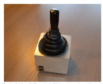
The joystick from KLAB can be built into any operator cabin. With Anybus CompactCom in place, it can communicate on PROFINET (and also any other network) which increases the potential market.
