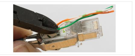
6. Press the wire block firmly into the connector assembly until it snaps into place.
