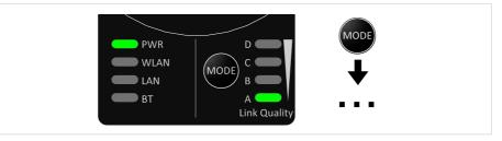
3. Press and hold **MODE** for 2 seconds to confirm Easy Config mode 1.
