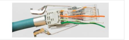
5. Press the shielding lugs together over the cable end to hold the connector in place and trim the wire ends close to the wire block.
