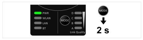
4. LED **A** will blink while the unit is scanning for the second unit.
