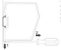
To unmount the device, use a screwdriver to push the DIN-rail fastening mechanism on the back of the device down until it locks in a fixed and open position (1). Then unhook the device from the DIN-rail (2).
