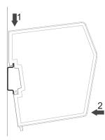
Ensure that the DIN-rail fastening mechanism on the back of the module is in a fixed and closed position, i. e. that it is pushed all the way up.
