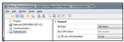
If the Control/Status Word is enabled no Bus Off Action can be defined.
