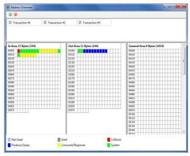
Note: The Address Overview is an offline tool with no reference to the module. It shows the memory usage of the the configuration that is present in the Anybus Configuration Manager at the moment.
