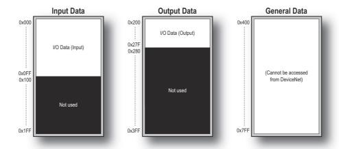
Please note that the two first bytes of the Output and Input Data areas are occupied by the Control/Status Word if this is enabled. Live List and Transmit and Receive Counters are by default mapped to the input memory area from the start address or after the Status Word.
