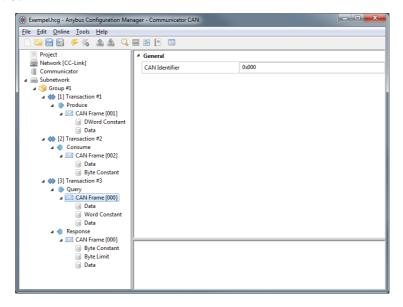
**Note**: A CAN frame can not contain more than 8 bytes of data. It is possible to configure the data area in each frame, but the size of the combination of objects must not exceed 8 bytes.
