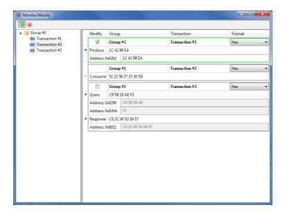
If Modify is enabled, it is possible to change the data values during runtime in Produce transactions and in the Query part of Query/Response transactions, i.e. only the out area of the Communicator can be modified. This will inhibit any data from the industrial network (PROFINET IO), but input data from the CAN network will still be updated.
