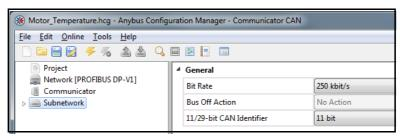
If the Control/Status Word is enabled no Bus Off Action can be defined.
