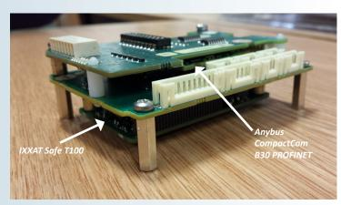
What safety looks like. The IXXAT Safe T100 implements the PROFIsafe layer and the safe control of three dual-channel inputs, as well as one dual-channel output. The Anybus CompactCom handles the unsafe communication and routes the safety communication to the IXXAT T100 via the black channel.
