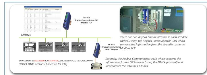
deemed that the Anybus Communicator CAN would be a perfect fit to handle the conversion between the CANbased network in the 22 straddle carriers and the Modbus-TCP network. The Anybus Communicator CAN works as a translator between the CAN-bus in the straddle carrier and the Modbus TCP of the communication system, converting each telegram through built-in hardware and software. Together with PICS, APM Terminals started mapping the communication between the CAN-bus and the monitoring system.
