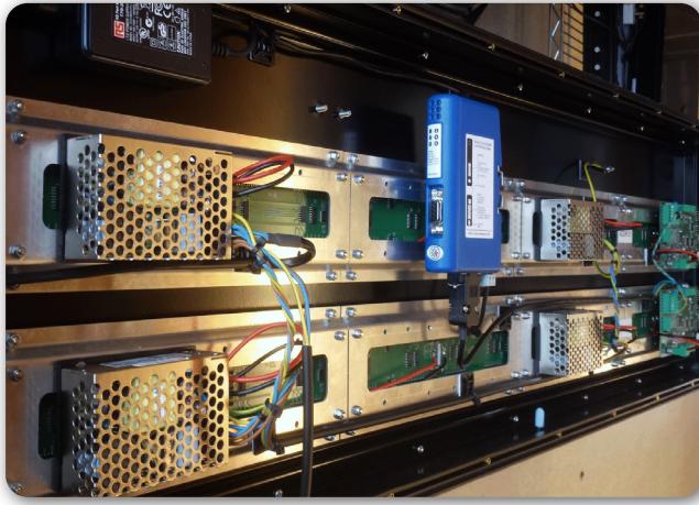
Behind the display. The Anybus Communicator in action inside one of London Electronics' displays, converting data from the PROFIBUS network to the display system.
