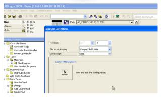
The configuration is integrated into Rockwell Studio5000. With a click of the mouse, you start the configurator for the Linking Device.
