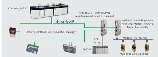
The EtherNet/IP to Serial Linking Device from HMS integrates industrial devices communicating via RS232/422/485, Modbus RTU and DF1 with a Rockwell PLC. You do all configuration in your familar Rockwell Studio 5000 environment.
