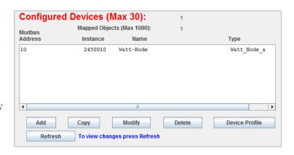
Pressing **Add, Copy** or **Modify** opens a new screen in which you can name the device and set its Modbus Address. Leave the Modbus IP Address at 0.0.0.0 to disable Modbus TCP for this device. A non-zero value assumes a Modbus TCP device and not a Modbus Serial device.
