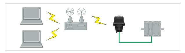
This example shows how to connect a PLC with an Ethernet network interface to an existing WLAN with support for layer 2 and layer 3 traffic. The WLAN interface in the Wireless Bolt will clone the MAC address of the Ethernet interface in the PLC.
