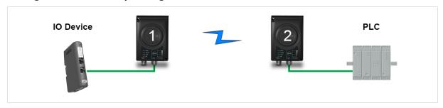
This example describes how to connect a PROFINET IO device and a PROFINET PLC over Bluetooth using two Wireless Bridges and Easy Config.
