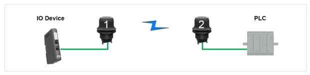
This example describes how to connect a PROFINET IO device and a PROFINET PLC over Bluetooth using two Wireless Bolts and Easy Config.
