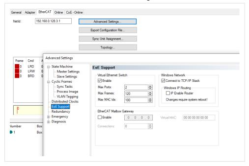
4. Generate an ESI-file for the slave and copy it to the 'C:\TwinCAT\3.1\Config\lo\EtherCAT' folder.
